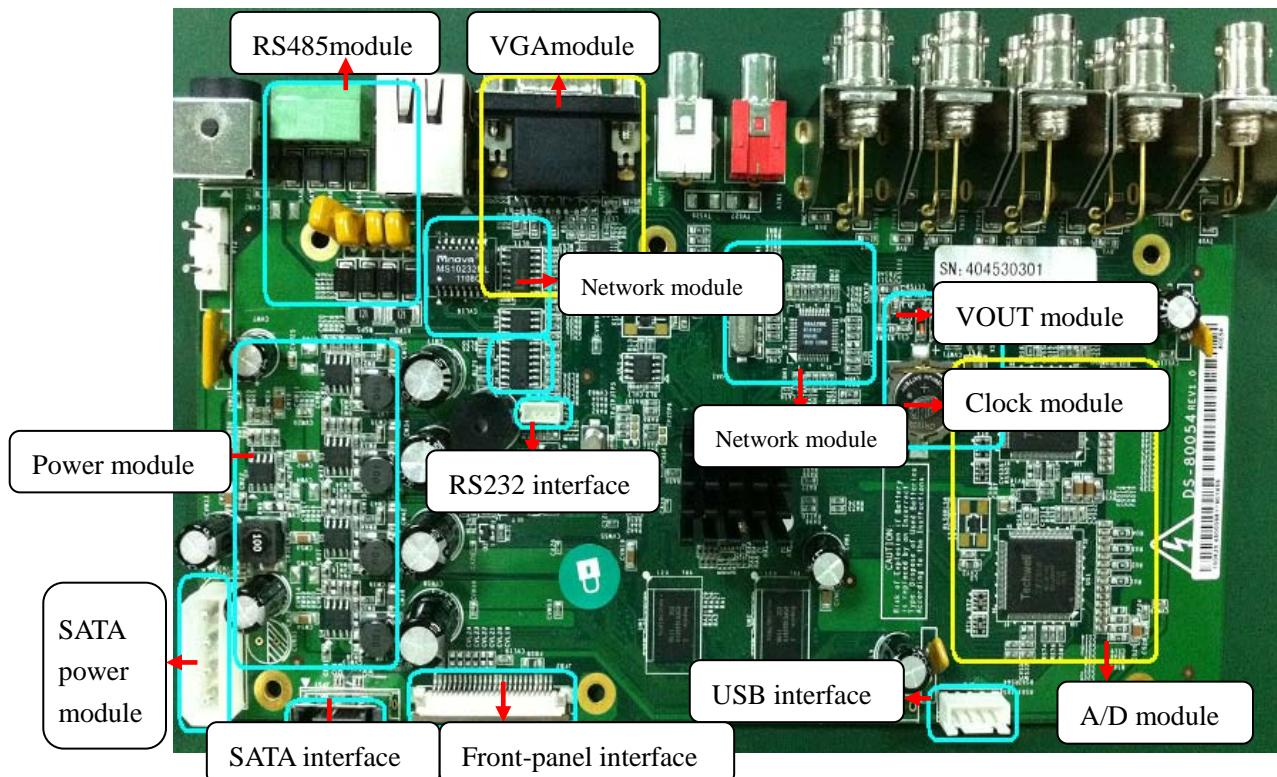
Diagram 1.2 DS80054 Mainboard Hardware Modules Diagram
